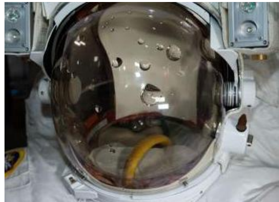
Figure 2. Water in helmet of EVA23 astronaut (MIB 2013)
